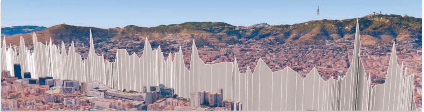
Signal coverage analysis performed along Barcelona Diagonal Avenue drawn as a curve depicting the power levels of a digital channel, showing Collserola emitting tower at the background.
